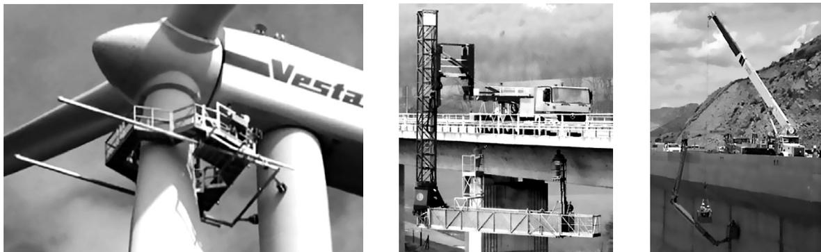
**Figure 1.** Conventional inspection units for large structures: elevating platform (left, Kaufer), underbridge unit (centre, WEMO-tec), truck crane (right, N.E. Bridge Contractors Inc.)
