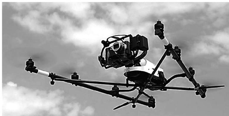
Figure 2. Flight system Falcon Photo with Panasonic Lumix TZ 22
