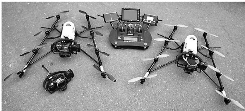
Figure 3. Flight systems with mobile ground station (remote control): Falcon Photo (left), Falcon Video (right)
